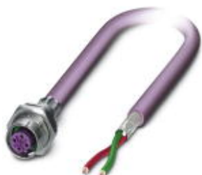
Bus system flush-type socket, PROFIBUS, 2-pos., M12, shielded, B-coded, SPEEDCON, rear/screw mounting with Pg9 thread, with 1.0 m bus cable, 2 x 0.25 mm 2
