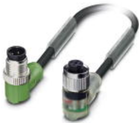
Sensor/actuator cable, 4-position, PVC, black RAL 9005, Plug angled M12, A-coded, on Socket angled M12, A-coded, with 3 LEDs, cable length: 0.3 m
