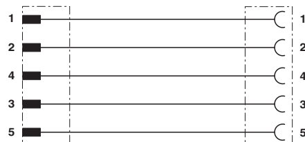
Contact assignment of M12 connector/socket
