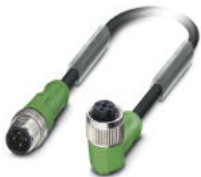
Sensor/actuator cable, 4-position, PVC, black RAL 9005, Plug straight M12, A-coded, on Socket angled M12, A-coded, cable length: 0.3 m
