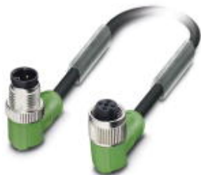
Sensor/actuator cable, 4-position, PVC, black RAL 9005, Plug angled M12, A-coded, on Socket angled M12, A-coded, cable length: 3 m
