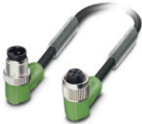
Sensor/actuator cable, 4-position, PVC, black RAL 9005, Plug angled M12, A-coded, on Socket angled M12, A-coded, cable length: 1.5 m
