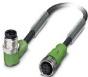
Sensor/actuator cable, 4-position, PVC, black RAL 9005, Plug angled M12, A-coded, on Socket straight M12, A-coded, cable length: 3 m
