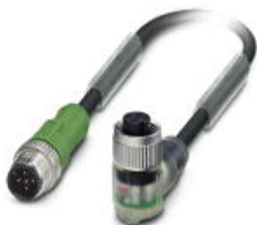
Sensor/actuator cable, 5-position, PVC, black RAL 9005, Plug straight M12, A-coded, on Socket angled M12, A-coded, with 3 LEDs, cable length: 0.6 m
