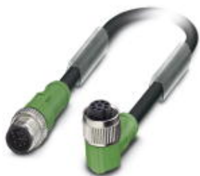
Sensor/actuator cable, 8-position, PVC, black RAL 9005, Plug straight M12, A-coded, on Socket angled M12, A-coded, cable length: 0.6 m
