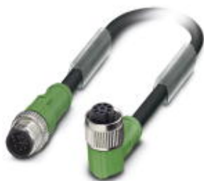
Sensor/actuator cable, 8-position, PVC, black RAL 9005, Plug straight M12, A-coded, on Socket angled M12, A-coded, cable length: 1.5 m
