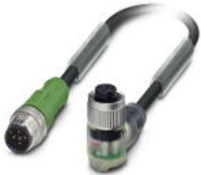
Sensor/actuator cable, 5-position, PVC, black RAL 9005, Plug straight M12, A-coded, on Socket angled M12, A-coded, with 3 LEDs, cable length: 0.3 m
