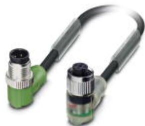
Sensor/actuator cable, 4-position, PVC, black RAL 9005, Plug angled M12, A-coded, on Socket angled M12, A-coded, with 3 LEDs, cable length: 3 m
