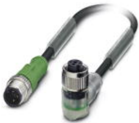
Sensor/actuator cable, 3-position, PUR, orange RAL 2003, Plug straight M12, A-coded, on Socket angled M12, A-coded, with 2 LEDs, cable length: 2 m
