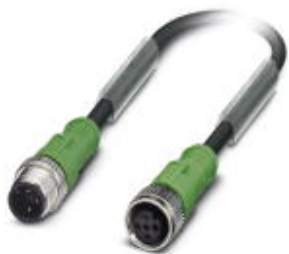
Sensor/actuator cable, 3-position, PVC, black RAL 9005, Plug straight M12, A-coded, on Socket straight M12, A-coded, cable length: 3 m
