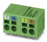
PCB terminal block, nominal current (Ex): 23 A, nominal voltage (Ex): 176 V, pitch: 5 mm, number of positions: 4, connection method: Push-in spring connection, mounting: Wave soldering, color: green. PCB terminal block satisfies the requirements of the "Guideline for PROFINET" in the edition dated 05/2017
