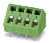
PCB terminal block, nominal current (Ex): 16 A, nominal voltage (Ex): 176 V, pitch: 5 mm, number of positions: 4, connection method: Spring-cage connection, mounting: Wave soldering, conductor/PCB connection direction: 45 °, color: green. PCB terminal block satisfies the requirements of the "Guideline for PROFINET" in the edition dated 05/2017
