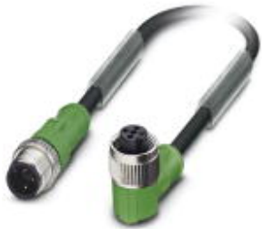
Sensor/actuator cable, 3-position, PVC, black RAL 9005, Plug straight M12, A-coded, on Socket angled M12, A-coded, cable length: 3 m
