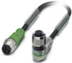
Sensor/actuator cable, 3-position, PVC, black RAL 9005, Plug straight M12, A-coded, on Socket angled M12, A-coded, with 2 LEDs, cable length: 0.6 m
