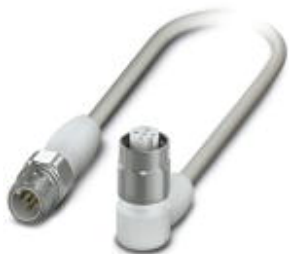
Sensor/actuator cable, 5-position, PP-EPDM halogen-free, gray RAL 7035, Plug straight M12, A-coded, on Socket angled M12, A-coded, cable length: 0.6 m, Hygienic design, with high-grade steel knurl
