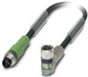
Sensor/actuator cable, 3-position, PVC, black RAL 9005, Plug straight M8, on Socket angled M8, with 2 LEDs, cable length: 0.6 m
