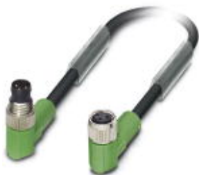
Sensor/actuator cable, 3-position, PVC, black RAL 9005, Plug angled M8, on Socket angled M8, cable length: 1.5 m
