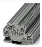
Double-level spring-cage terminal block, connection method: Spring-cage connection, cross section: 0.08 mm² - 4 mm², AWG: 28 - 12, width: 5.2 mm, color: gray, mounting type: NS 35/7,5, NS 35/15
