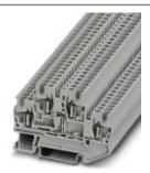
Double-level spring-cage terminal block, connection method: Spring-cage connection, cross section: 0.08 mm² - 1.5 mm², AWG: 28 - 16, width: 4.2 mm, color: gray, mounting type: NS 35/7,5, NS 35/15
