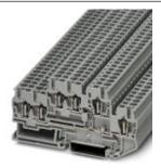
Double-level spring-cage terminal block, connection method: Spring-cage connection, cross section: 0.08 mm² - 4 mm², AWG: 28 - 12, width: 5.2 mm, color: gray, mounting type: NS 35/7,5, NS 35/15
