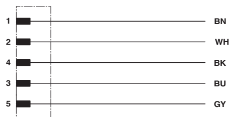
Contact assignment of the M12 socket
