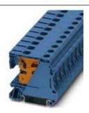
N disconnect terminal block, for neutral conductor disconnection, Screw connection, cross section: 6 mm² - 25 mm², AWG: 10 - 4, width: 12.2 mm, color: blue, mounting type: NS 35/7,5, NS 35/15
