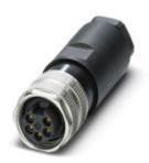
Connector, 5-position, Socket straight 7/8"-16UNF, Screw connection, knurl material: Zinc die-cast, nickel-plated, cable gland Pg13,5, external cable diameter 10 mm ... 12 mm
