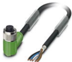
Sensor/actuator cable, 5-position, PUR halogen-free, black-gray RAL 7021, shielded, free cable end, on Socket angled M12, A-coded, cable length: 10 m
