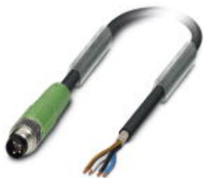
Sensor/actuator cable, 4-position, PUR halogen-free, black-gray RAL 7021, shielded, Plug straight M8, on free cable end, cable length: 5 m
