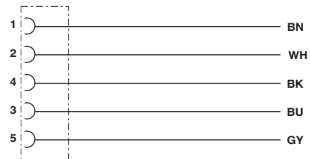
Contact assignment of the M12 socket
