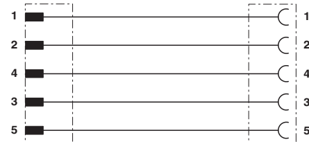
Contact assignment of the M12 connector and the M12 socket
