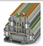
Knife disconnect terminal block, With test socket screws for insertion of test plugs, nom. voltage: 400 V, nominal current: 16 A, connection method: Screw connection, cross section: 0.14 mm² - 4 mm², AWG: 26 - 12, length: 80.1 mm, width: 5.2 mm, color: gray, mounting: NS 35/7,5, NS 35/15, nom. voltage: 400 V
