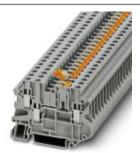
Knife disconnect terminal block, With test socket screws for insertion of test plugs, nom. voltage: 500 V, nominal current: 20 A, connection method: Screw connection, number of connections: 3, cross section:0.14 mm² - 6 mm², AWG: 26 - 10, width: 6.2 mm, color: gray, mounting type: NS 35/7,5, NS 35/15
