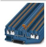
Knife disconnect terminal block, nom. voltage: 400 V, nominal current: 16 A, connection method: Push-in connection, cross section: 0.14 mm² - 4 mm², AWG: 26 - 12, length: 92.2 mm, width: 5.2 mm, color: blue, mounting: NS 35/7,5, NS 35/15, nom. voltage: 400 V
