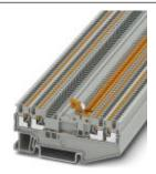
Knife disconnect terminal block, nom. voltage: 400 V, nominal current: 10 A, connection method: Push-in connection, cross section: 0.14 mm² - 1.5 mm², AWG: 26 - 14, length: 76.9 mm, width: 3.5 mm, color: gray, mounting: NS 35/7,5, NS 35/15, nom. voltage: 400 V
