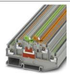
Knife disconnect terminal block, nom. voltage: 400 V, nominal current: 9 A, connection method: Push-in connection, cross section: 0.14 mm² - 1.5 mm², AWG: 26 - 14, length: 86 mm, width: 3.5 mm, color: gray, mounting: NS 35/7,5, NS 35/15, nom. voltage: 400 V
