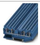
Feed-through terminal block, nom. voltage: 800 V, nominal current: 32 A, connection method: Spring-cage connection, number of connections: 4, cross section:0.08 mm² - 6 mm², AWG: 28 - 10, width: 6.2 mm, color: blue, mounting type: NS 35/7,5, NS 35/15
