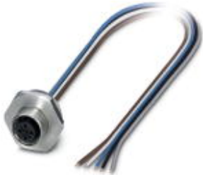
Sensor/actuator flush-type socket, 4-pos., M12, A-coded, front/screw mounting with M20x1.5 thread, with 0.5 m TPE litz wire, 4 x 0.34 mm 2 , stainless steel design
