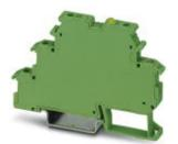
Power solid-state relay terminal block, input: 5 V DC, output: 10 - 253 V AC/800 mA, terminal block width: 6.2 mm
