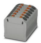
Distribution block, internally jumpered, connection method: Push-in connection, number of connections: 12, cross section:0.14 mm² - 1.5 mm², AWG: 26 - 16, width: 25.2 mm, height: 17.6 mm, color: gray, mounting type: Direct mounting with flange
