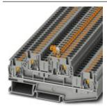
Knife disconnect terminal block, connection method: Push-in connection, cross section: 0.2 mm<sup>2</sup> - 6 mm<sup>2</sup>, AWG: 24 - 10, length: 102.9 mm, width: 6.2 mm, color: gray, mounting: NS 35/7,5, NS 35/15
