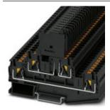
Fuse modular terminal block, connection method: Push-in connection, cross section: 0.2 mm²- 6 mm², AWG: 24 - 10, nominal current: 28 A, nom. voltage: 500 V, width: 6.2 mm, fuse type: G / 5 x 20, fuse type: Glass / ceramics / ..., mounting type: NS 35/7,5, NS 35/15, color: black
