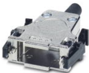
D-SUB sleeve housings, Degree of protection: IP20, Material: Zinc die-cast, Cable exit: straight, Size of housing: 2, Color: Bare metallic, Snap-fit locking
