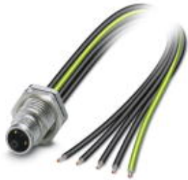
Flush-type connector, Power, 5-position, Plug, M12, K - Power, Rear mounting, M16 x 1.5, Individual wires, Cable length: 0.2 m
