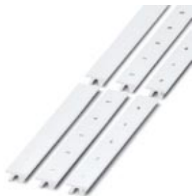
Zack marker strip, Strip, white, labeled, Printed horizontally: L1, L2, L3, N, PE, Mounting type: Snap into tall marker groove, for terminal block width: 16.3 mm, Lettering field: 10.5 x 16.25 mm
