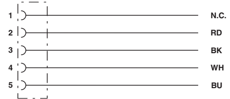
Contact assignment of 7/8" socket
