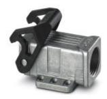
Box mounting bases D7, With single locking latch, Material: Die-cast aluminum, salt water resistant, Cable outlets: 1, lateral, Height: 27.9 mm, Cable gland: none, Gland: Yes, 1x Pg11, Standard, enclosed bottom
