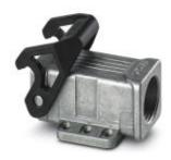
Box mounting bases D7, With single locking latch, Material: Die-cast aluminum, salt water resistant, Cable outlets: 1, lateral, Height: 27.9 mm, Cable gland: none, Gland: Yes, 1x M20, Standard, open floor
