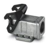
Box mounting bases D7, for single locking latch, Material: Die-cast aluminum, salt water resistant, Cable outlets: 1, lateral, Height: 27.9 mm, Cable gland: none, Gland: Yes, 1x Pg11, Standard, open floor
