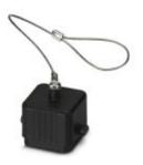
Protective cover D7, for single locking latch, Material: PA, Protective cover material: PA, Height: 29.4 mm, Seal: yes, Standard, With lanyard, Diameter of retaining cord eyelet: 25 mm, for socket inserts
